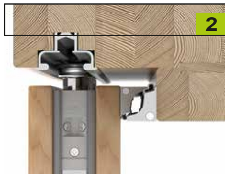
FLUSH GUIDE RAIL WITH ROLLER GUIDE for uniquely smooth-running sliding comfort
